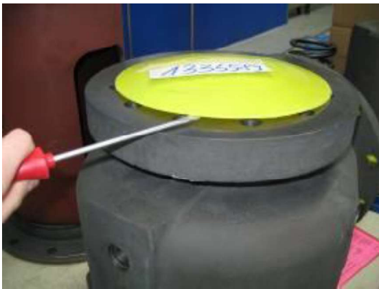
Fig. 3 Lifting the protective cap
